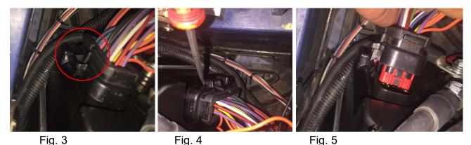
10. Remove the remaining cabling; pack negative cable and the three motor cables from the controller and move them up and out of the way.
